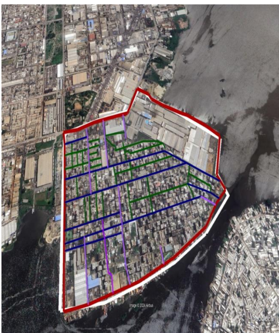
FIGURE 1 SOWETO NETWORK DESIGNED
