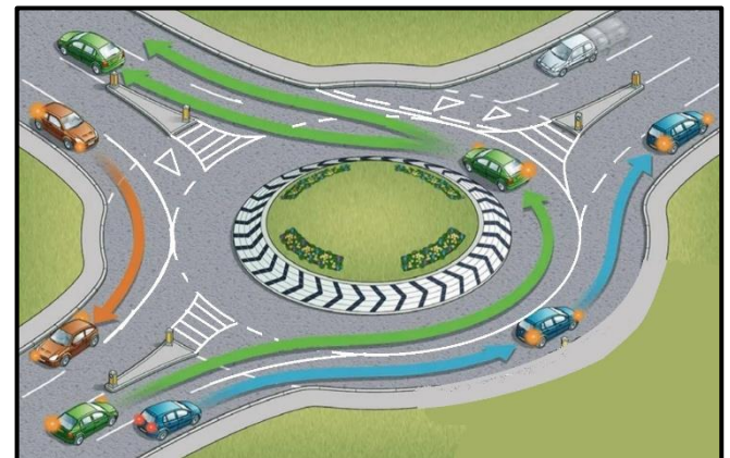
Fig. 16. Lane alignment through a "turbo lane", entry and traffic flow at a three way roundabout [7].
