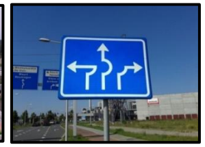
Figure 20. Road sign to indicate that you are in the appropriate lane in a turboroundabout [11].
