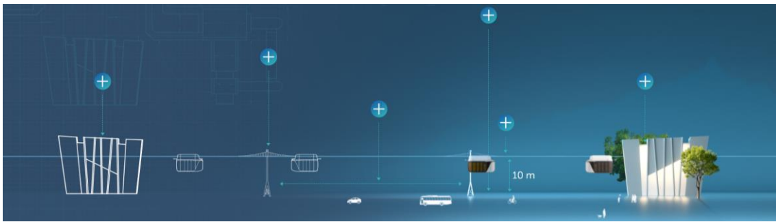
Figure 3. Schematic representation of the composition of the uST complex (anchor support, intermediate support, unimobile, anchor support combined with passenger station)
