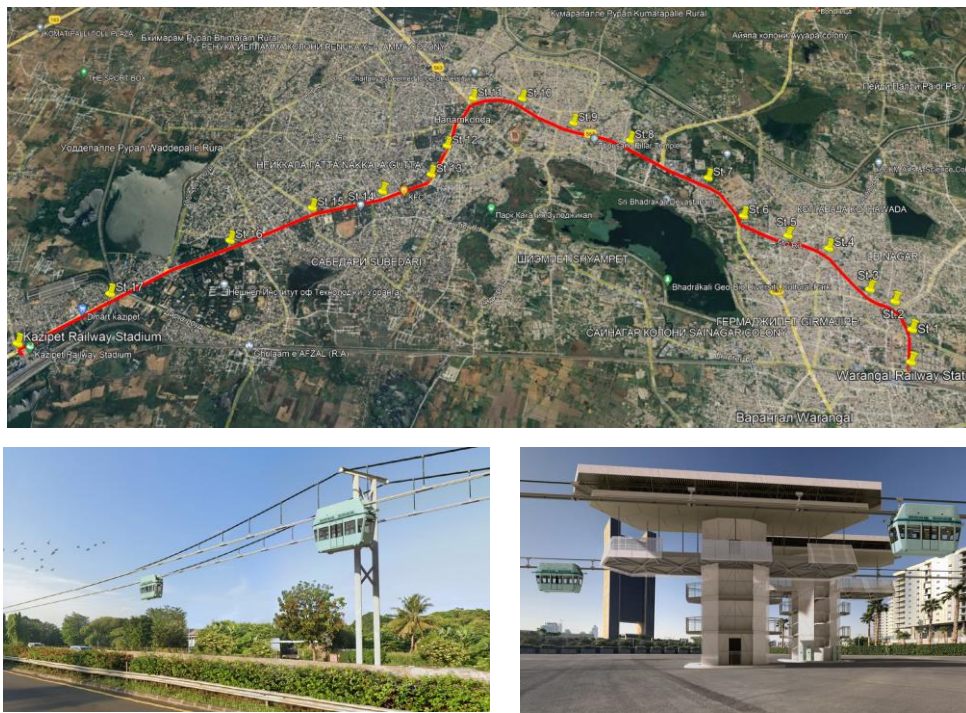
Figure 6. Design visualization option of Warangal-Hanamkonda-Kazipet suspension type uST route network with length of 15 km Source: authors' elaboration
