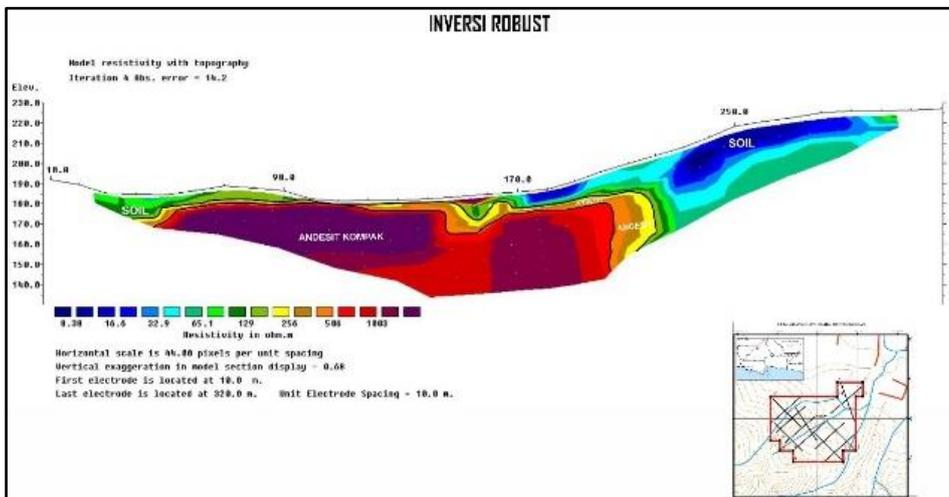
Figure 5. Inversion modeling results with Robust inversion of line 1
