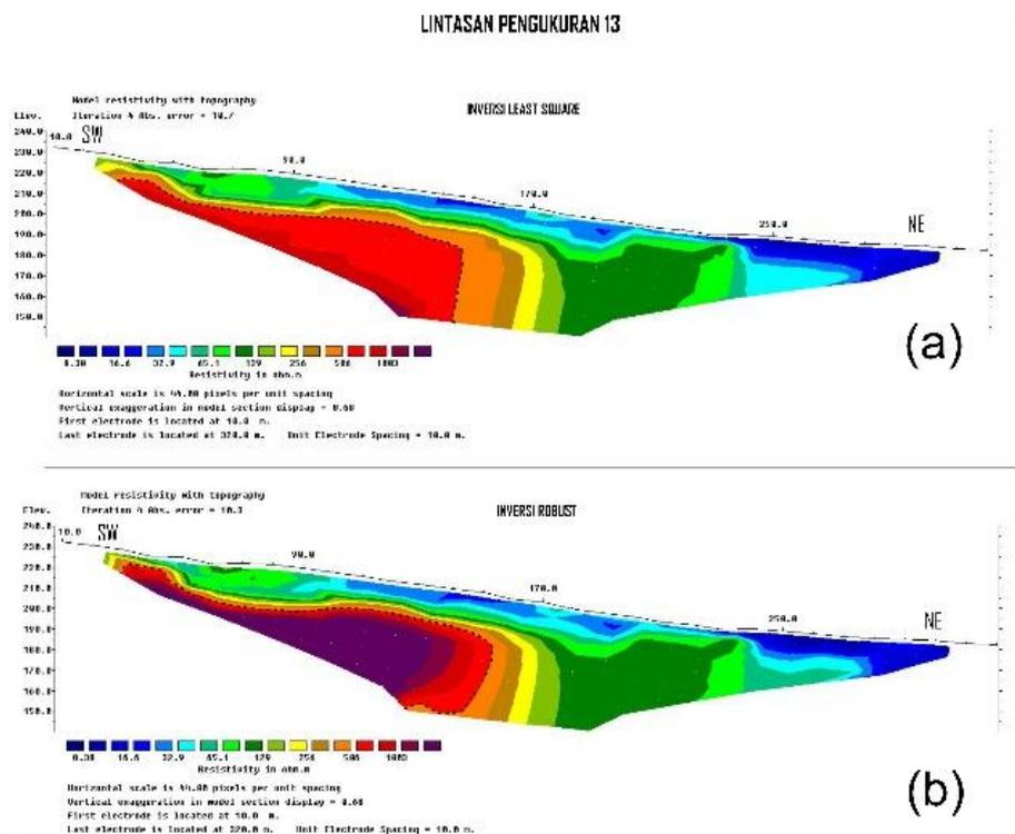
**Figure 3** Results of Least Square Inversion and Robust Inversion. (a) Least Square inversion method (b) Robust inversion method Line 13
