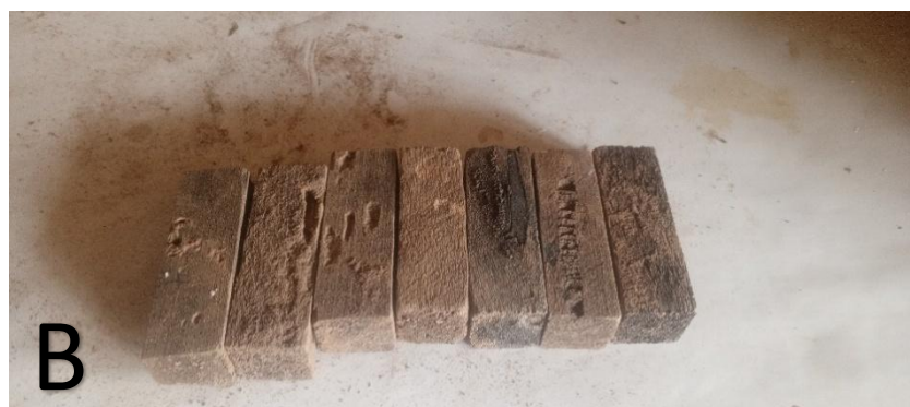
Plate 1: Effects of Termite attack on the wood specie. A: Sound samples of Terminalia superba after exposure to Termite Attack for 12 weeks, B: Slightly attacked samples of Triplochyton scleroxylon after exposure to termite attack for 12 weeks
