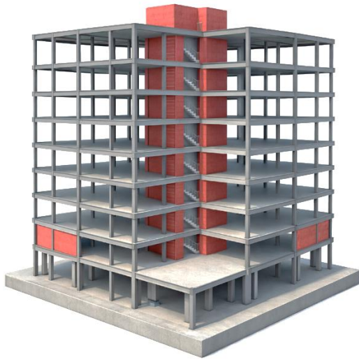
Figure 1. Three-dimensional structural model of the reference mid-rise building illustrating the lateral load-resisting system used in the STRIDE coupled dynamic–energy analysis.
