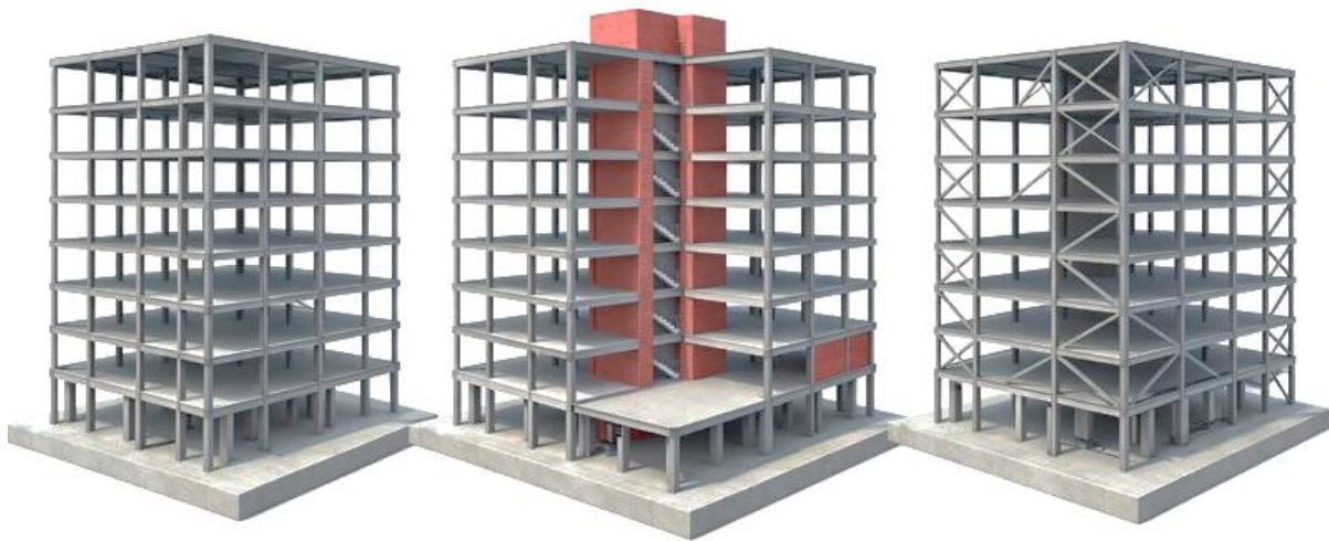
Figure 2. Comparative three-dimensional structural models representing different lateral load-resisting systems under identical geometric and boundary conditions.
