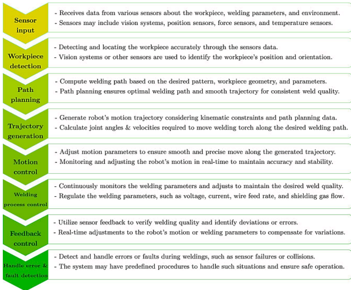
Figure 1: General process involved in control systems of welding robots, [14].
